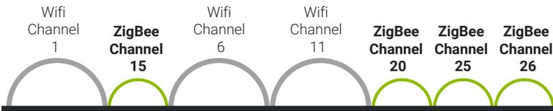
The foundation of every ZigBee standard and specification is the powerful IEEE 802.15.4 physical radio standard, which operates in unlicensed bands worldwide at 2.4GHz (global), 915Mhz (Americas) and 868Mhz (Europe). The ZigBee standard offers reliable communications of information packets with excellent data throughput rates of 250Kbs at 2.4GHz (16 channels), 40Kbs at 915Mhz (10 channels) and 20Kbs at 868Mhz (1 channel).
